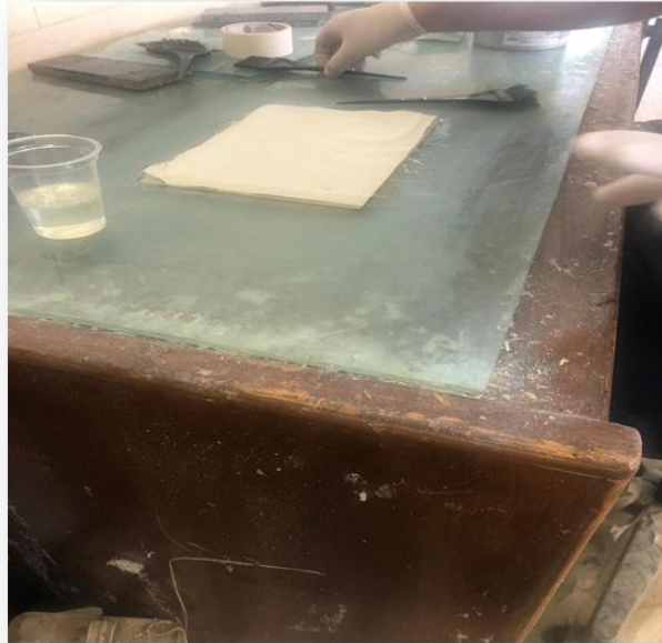
6 layers cotton with epoxy
