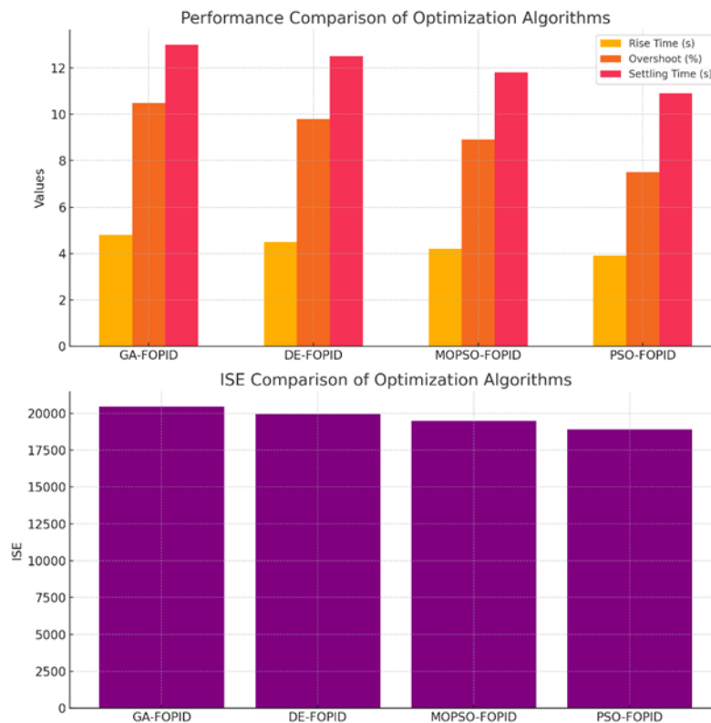
Figure 8. Comparative performance of GA, DE, MOPSO, and PSO in terms of rise time, overshoot, settling time, and ISE, highlighting the superior effectiveness of PSO-FOPID.
