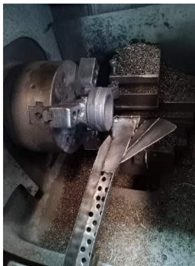
Gambar 6. Proses Potong Material
