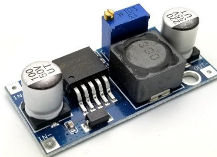
Figure 4: shown a DC to DC voltage regulator
