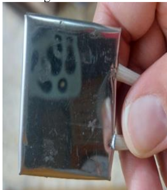
(Figure 6) shows the electrical heater.
