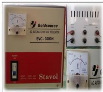
(Figure 9) shows the Voltage regulator
