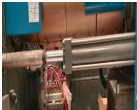
Gambar 4. Silinder Hidrolik Mesin Injection Molding
